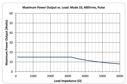
Figure 9-2 Maximum Power Output for Mode 10 Pulse
