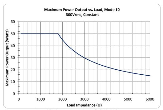
Figure 9-1 Maximum Power Output for Mode 10 Constant
