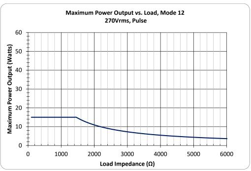
Figure 9-4 Maximum Power Output for Mode 12 Pulse
