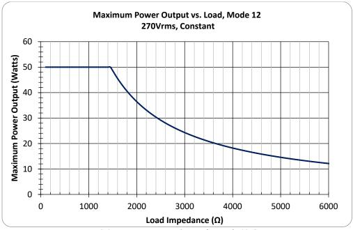
Figure 9-3 Maximum Power Output for Mode 12 Constant
